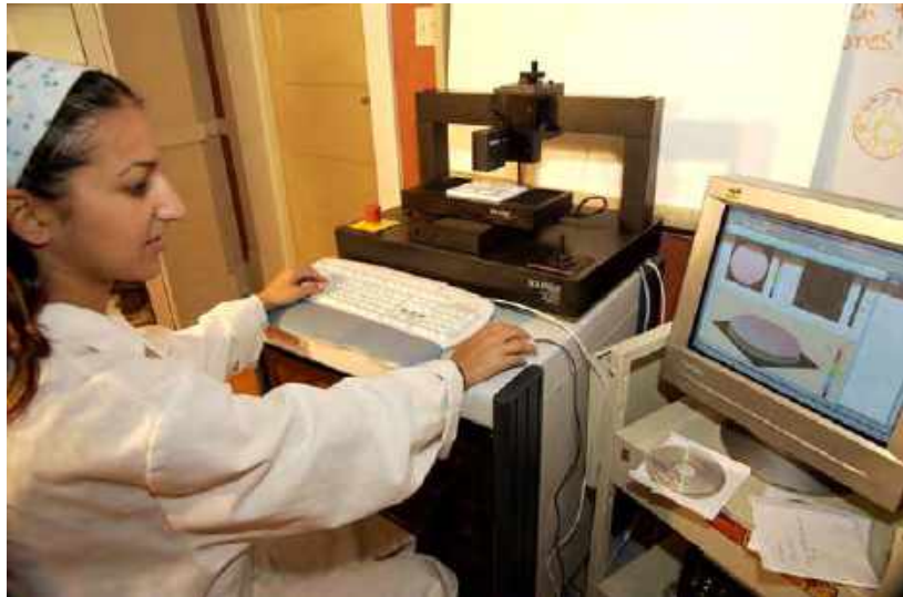
Figure 15. Researcher scans surface of stone using laser profilometer to determine texture parameters and 3-d profile.
