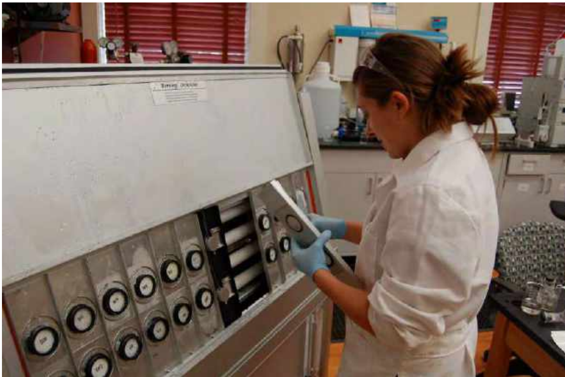
Figure 11. Marble samples being removed from the QUV weatherometer during a dark cycle to be treated with cleaner.
