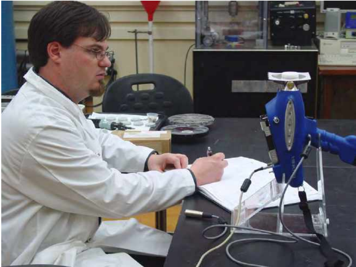
Figure 12. Jason Church uses the XRF spectrometer to analysis a marble sample after artificial weathering.
