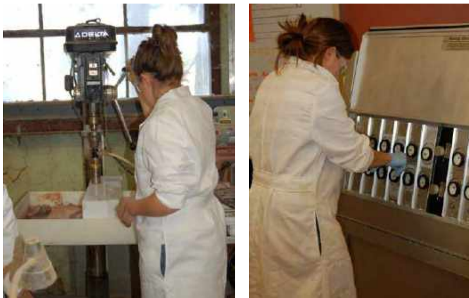
Figure 17. On right samples are cored from Colorado Yule Marble. On left samples are placed into QUV weathering tester.
