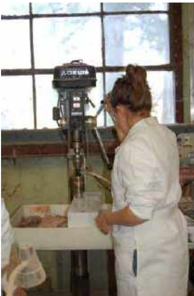
Figure 10. Georgette Lang cores a sample of Colorado Yule for use in the accelerated weathering study.
