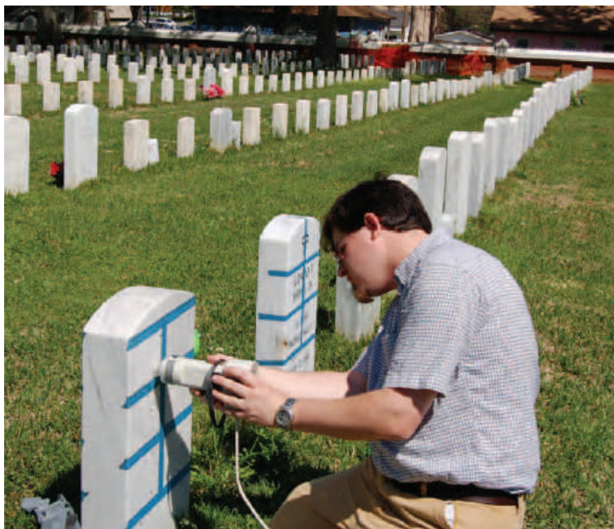
FIGURE 1. Jason Church takes color measurements of a headstone after cleaning.
