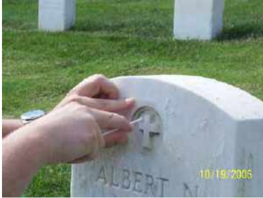
Figure 3. Photographic detail showing an acetate template being used as a guide for swabbing the headstone.
