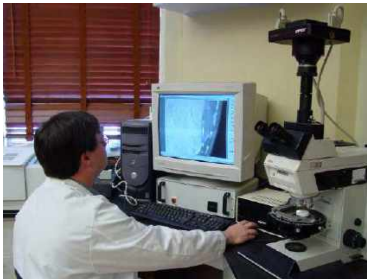
Figure 16. Jason Church uses an optical microscope fitted with a digital Spot camera to view salt deposits on the back of a sample
