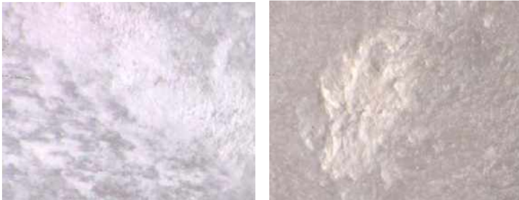
Figure 1. These images were gathered from field samples placed in the cemetery during field trials. The micrograph on the left shows possible salts from D/2 cleaning collecting on the surface of a Colorado Yule sample. The micrograph on the right show possible salts from Daybreak within a pore of the stone. All micrographs were taken at 25X magnification.
